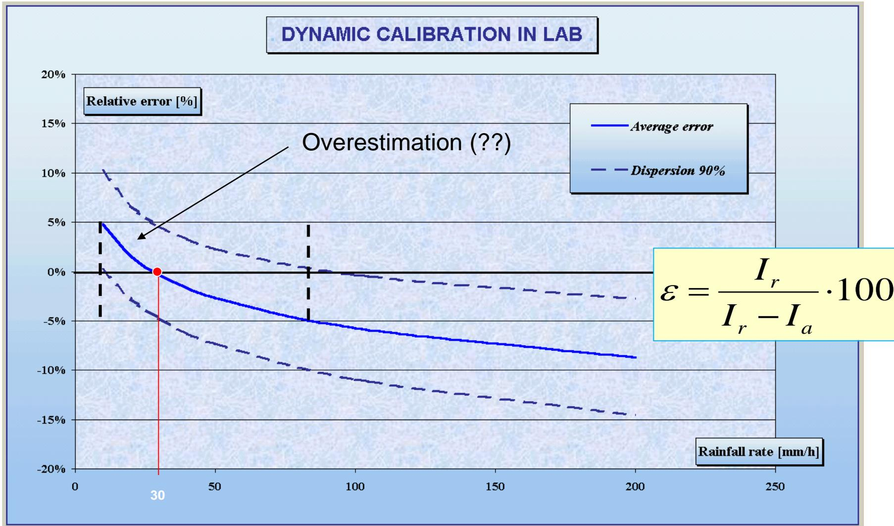
(about 60 instruments, various models, used at the former Hydrographic Service of Genoa - Italy)
