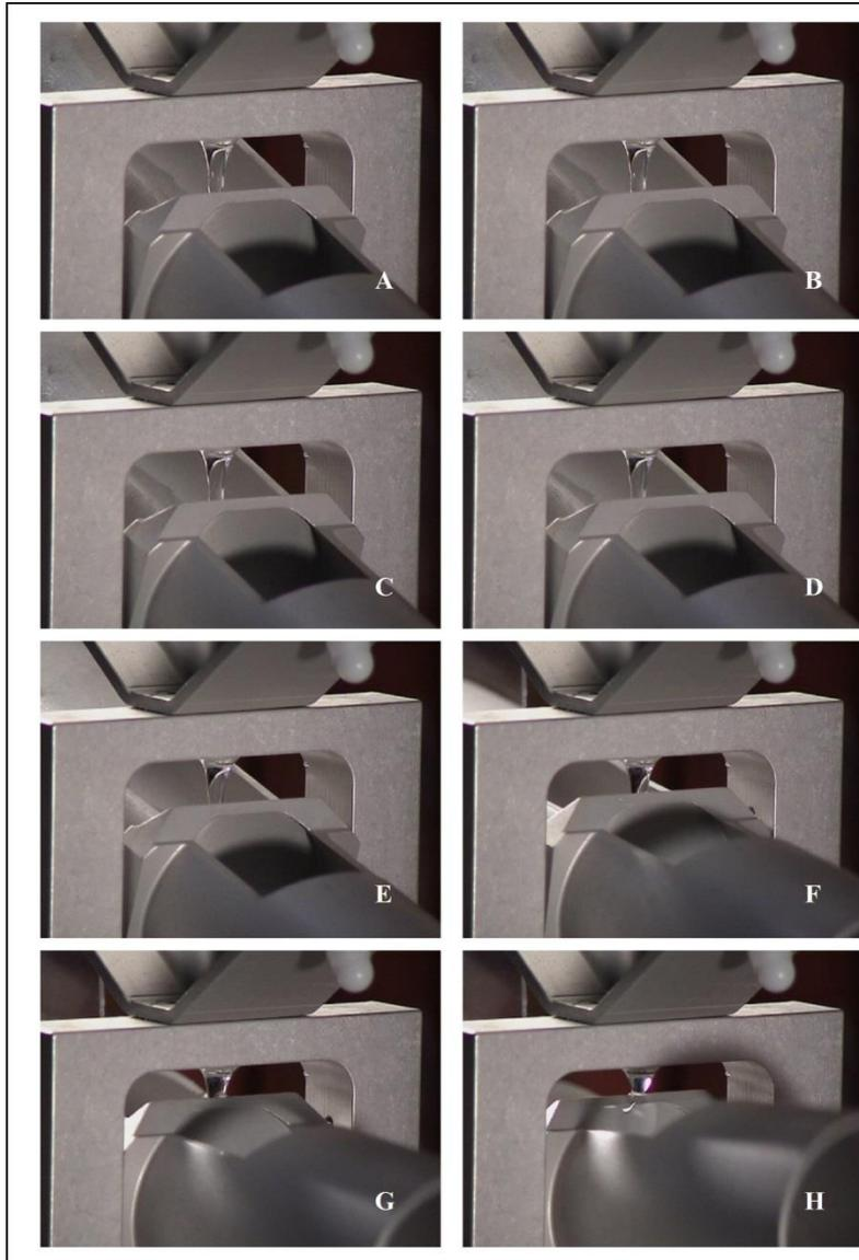
The **measurement of rainfall intensity**, traditionally performed by means of tipping bucket rain gauges is therefore **subject to a systematic underestimation of high rain rates** due to the amount of water lost during the tipping movement of the bucket.
